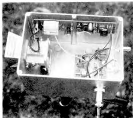
The complete 10GHz transceiver showing the Solfan horn aerial as supplied.
