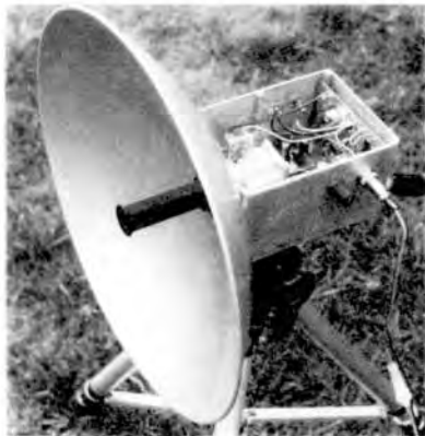
A general view of the transceiver fitted with a dish aerial and 'penny' feed (see RSGB VHF/UHF Manual).
